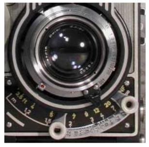
Shutter is a Metax, B, and 1-400 speed with self-timer and X flash synch. The focus lever (which operates similar to the Minolta Autocords) has a depth of field indicator built into it.
